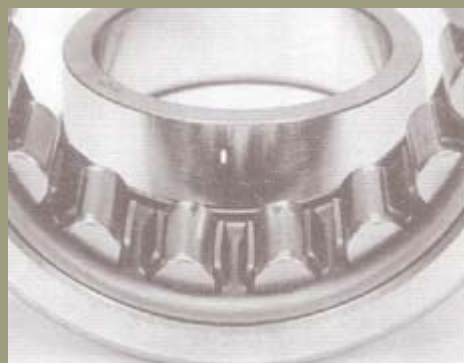
Cylindrical roller bearing with streaks on the rolling raceway of the inner ring and on the rollers due to wrong assembling operations.
