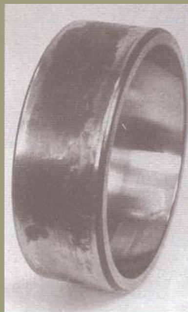
Contact rust ("fretting corrosion") on the outer ring of an adjustable bearing.
