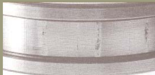
Inner ring of a cylindrical roller bearing damaged by vibrations. The damages occurred when the bearing was not rotating. It is clear, by seeing the littlest tracks between the more marked tilts (with corrosion on the bottom), that the ring has changed its position for small periods
