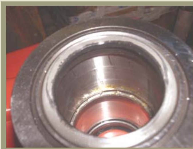
Bearing damaged on the guide brims and on the raceways of the outer ring, due to the axial thrusts.
