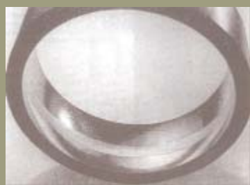
Outer ring of an adjustable roller bearing not adequately lubricated; the raceways are polished.
