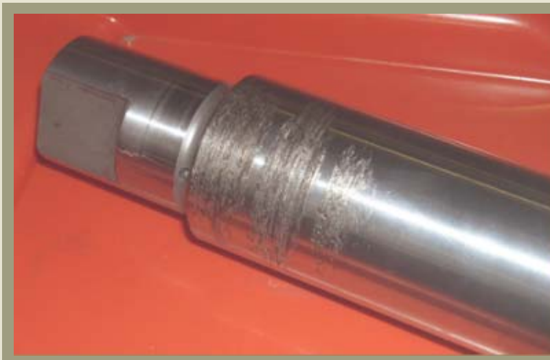
Pivot with marks of damages due to a non correct alignment; the part of the pivot which is not damaged is still polished.
