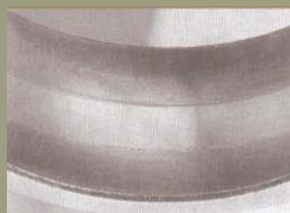
Outer ring of an revolving roller bearing with raceways worn by abrasive particles. It is easy to see the border between worn part and entire part.
