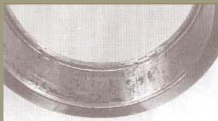
Deep rust on the outer ring of a cylindrical roller bearing.
